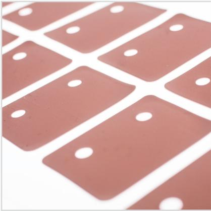
Keratherm brown, with its very good thermal properties, is an excellent choice for cost-effective solutions. These fibre glass reinforced films, along with their very smooth surface, have very good thermal resistance with a high insulation capacity at low mounting pressures.
