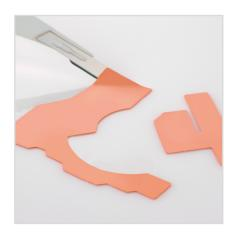
Softtherm 86/125 has an improved thermal performance without influencing the dielectric and mechanical properties. 86/125 is a single layer, supported with fibre glass reinforcement.
