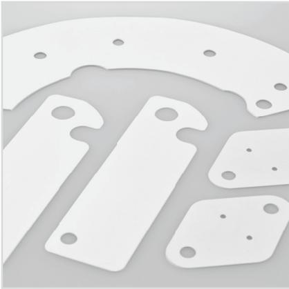
The highly thermoconductive white group, with its well-balanced thermal, electrical and dielectric behaviour and very good self-adhesion characteristics, is created by filling a silicone elastomer base with aluminum oxide. An increase in mechanical strength can be achieved through fibre glass reinforcement. These film types can optionally be supplied with an additional adhesive coating.
