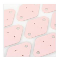
Keratherm pink offers outstanding thermal conductivity, which is achieved by a specially filled silicone elastomer. The good electrical insulation properties are thereby retained. On request, these films can also be supplied with fibre glass reinforcement and with or without adhesive coating. The excellent thermal resistance of this film enables the optimum heat transfer to the heat sink.
