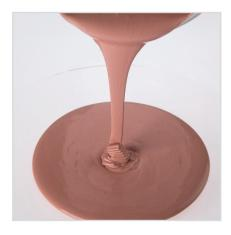
Ceramic-filled, solvent-free two-component silicone elastomers. Because of their various conductivities, their good dielectric properties and their compressibility characteristics, these Gapfillers are ideallysurtable for encapsualting or dispensing. A wide range of different material viscosities make them suitable for "wet-in-wet" production. Customized solutions for the compound and processing technology available.
