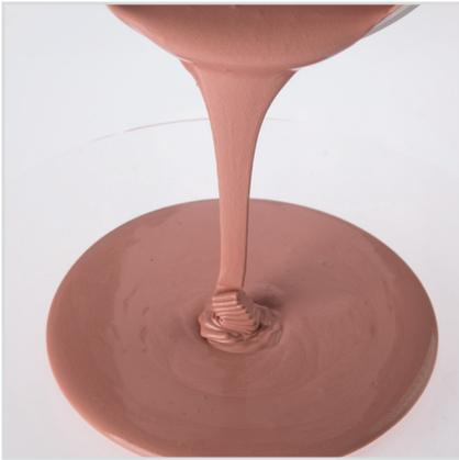
Ceramic-filled, solvent-free two-component silicone elastomers. Because of their various conductivities, their good dielectric properties and their compressibility characteristics, these Gapfillers are ideally suitable for encapsulating or dispensing. A wide range of different material viscosities make them suitable for "wet-in-wet" production. Customized solutions for the compound and processing technology available.
